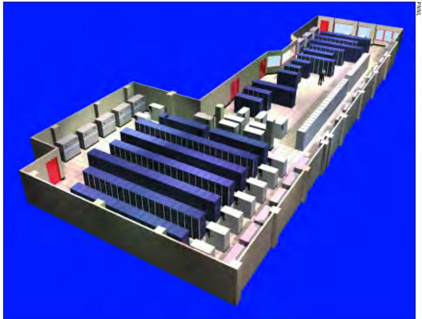
**Figure 2.** A three-dimensional rendition of the Chinook supercomputer at EMSL.
