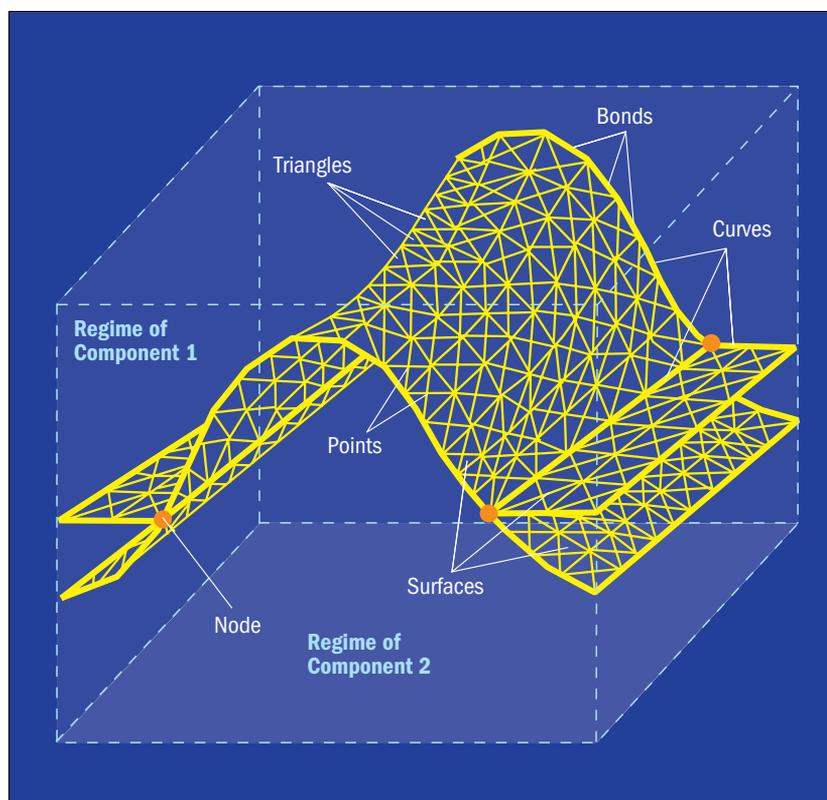
**Figure 8.** A triangular mesh representing the interface between two different materials. This mesh is moved through the computational domain to follow the motion of the interface.
