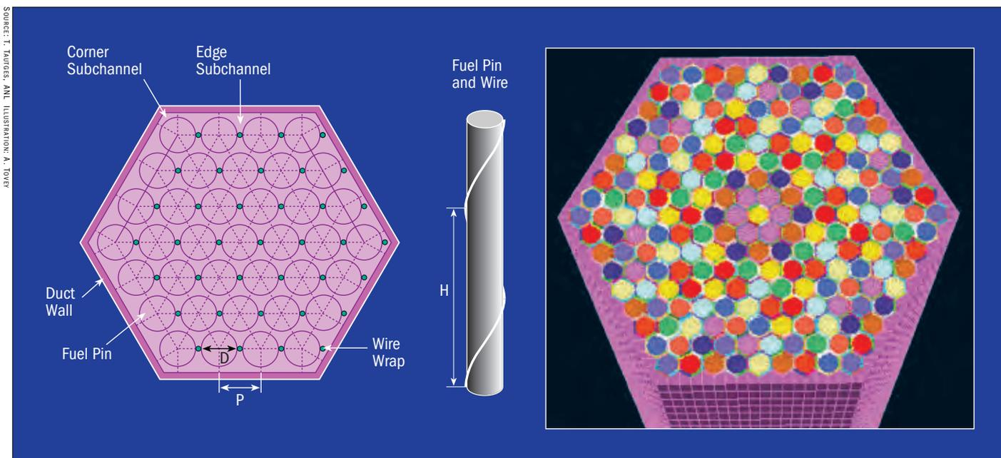
**Figure 15.** The geometrical domain and a conformal hexahedral mesh for modeling the reactor core of a sodium fast reactor.
