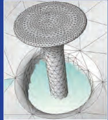
**Figure 12.** The curved geometries and high-order methods used by SLAC to model next-generation accelerators require that the meshes also be curved to achieve high accuracy. We have developed automatic procedures to locate and correct inverted elements which significantly improves simulation accuracy and efficiency.
