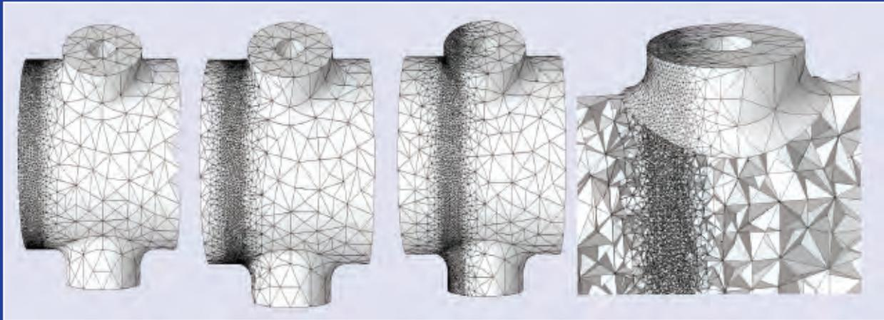
**Figure 13.** The left three images show the adapted mesh for following particles in an accelerator cavity at three points in time. The right-hand image shows a cut on the interior of the mesh.
