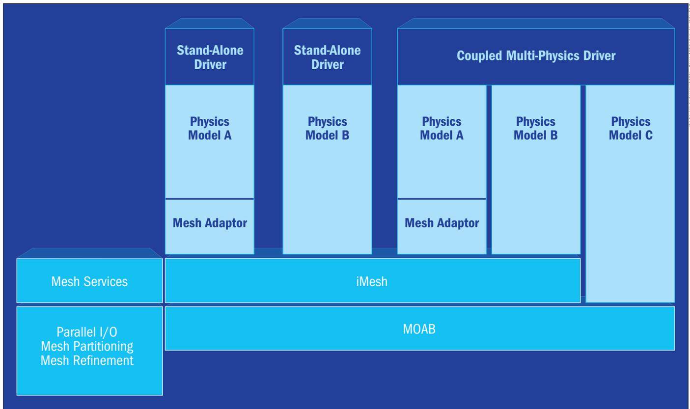
**Figure 16.** The SHARP framework developed at Argonne National Laboratory uses the ITAPS interfaces and tools as a key mechanism for coupling different physics modules together to perform high-fidelity simulations of nuclear reactors.
